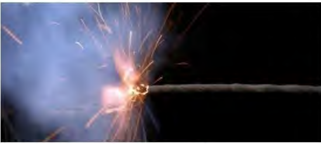
Detonating cord burning in one direction.
